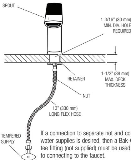
If a connection to separate hot and cold water supplies is desired, then a Bak-Chek® tee fitting (not supplied) must be used prior to connecting to the faucet.
