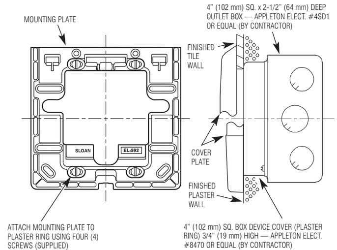
To ensure a perfect rough-in, Sloan recommends the use of the EL-485-A Flushometer Electrical Box Positioning and Support Kit. Specify and order the EL-485-A Kit separately. When using the EL-485-A kit, the Solenoid Plate roughs in at the Urinal location. Consult factory for installation details.
