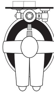
3. When the user steps away from the OPTIMA Sensor, the circuit waits 3 seconds (to prevent false flushing) then initiates an electrical "one-time" signal that operates the Solenoid. This initiates the flushing cycle to flush the fixture. The Circuit then automatically resets and is ready for the next user.
