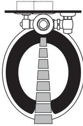
2. As the user enters the beam's effective range (22" to 42") the beam is reflected into the OPTIMA Scanner Window and transformed into a low voltage electrical circuit. Once activated, the Output Circuit continues in a "hold" mode for as long as the user remains within the effective range of the Sensor.
