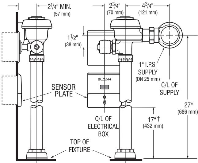
† Position of Sensor Box can be raised or lowered 1" (25 mm) if in conflict with Handicap Grab Bars.
