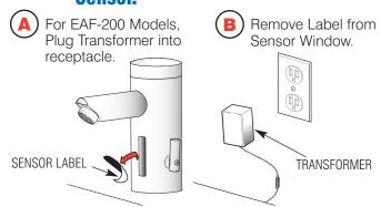
Electrical Connection for up to Six (6) Faucets Using One (1) Transformer
