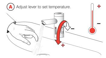
**Optional** — To fix temperature, set lever to the desired position, then remove lever and plug hole with Cap.
