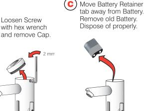
Insert a new 6 Volt Type CR-P2 Lithium Battery. The red LED will flash for one (1) minute. Reinstall Battery Cover. If LED doesn't flash or if it just lights up, remove and then reinsert the Battery. If water flows continuously after inserting the new Battery and opening the Supply Stops, remove and then reinsert the Battery.
