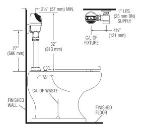
The Model 8116 valve is designed for installations where the water supply is roughed-in 27" (686 mm) above the top of the water closet. For new installations, Sloan strongly recommends the use of our Model 8111 which has a shorter installation height.
