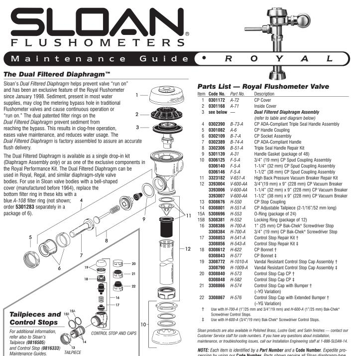
cessing by using our **Code Numbe**r. Parts shown service all Sloan diaphragm-type Flushometers manufactured after 1964, including Low Consumption (LC) models.
