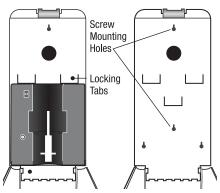
Install provided anchors into drywall and secure the dispenser with the provided screws. Replace battery compartment.
