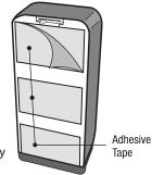
mounting surface for about 15 seconds. Open front cover and press directly against back plate for an additional 15 seconds. Allow 4 hours to set before using the dispenser.
