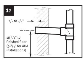
Set drain line height at 16  $^{3}/_{4}$ " from finished floor (standard 24" rim) or  $9^{3}/_{4}$ " for ADA installation. Threaded nipple should extend  $\frac{1}{2}$  to  $\frac{3}{4}$ " from wall.
