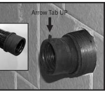
Apply lubricant to the outside of the rubber bushing and ribbed inside area. Insert the tube and bushing with the arrow tab at the top.
