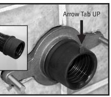
Apply lubricant to the outside of the rubber bushing and ribbed inside area. Insert the tube and bushing with the arrow tab at the top. Lube tailpipe of housing.
