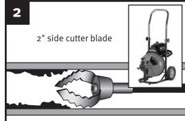
**IMPORTANT:** Use a drain machine to remove build-up inside pipes. Clean 25-35 feet deep then flush with water to remove cutting debris.
