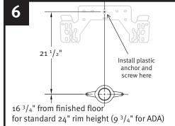
a 5/16" masonry bit to drill hole, then install the hanger bracket with one plastic anchor and screw.
