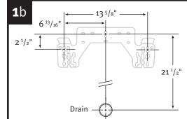
Carrier stud placement: If using inwall carrier, set bearing rods as shown above.
