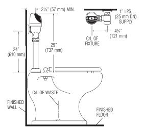
The Model 8115 valve is designed for installations where the water supply is roughed-in 24" (610 mm) above the top of the water closet. For new installations, Sloan strongly recommends the use of our Model 8111 which has a shorter installation height.
