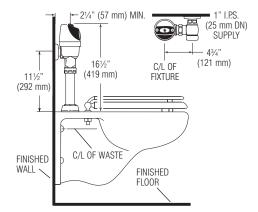
When installing the G2 Optima Plus in a handicap stall:
